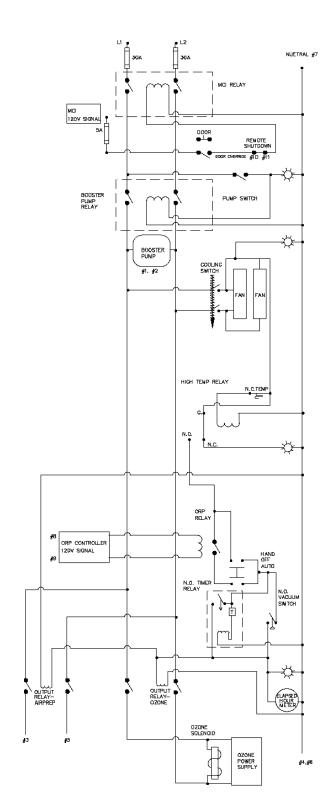
Shown: Electrical Schematic - CD-4000 Line Side
