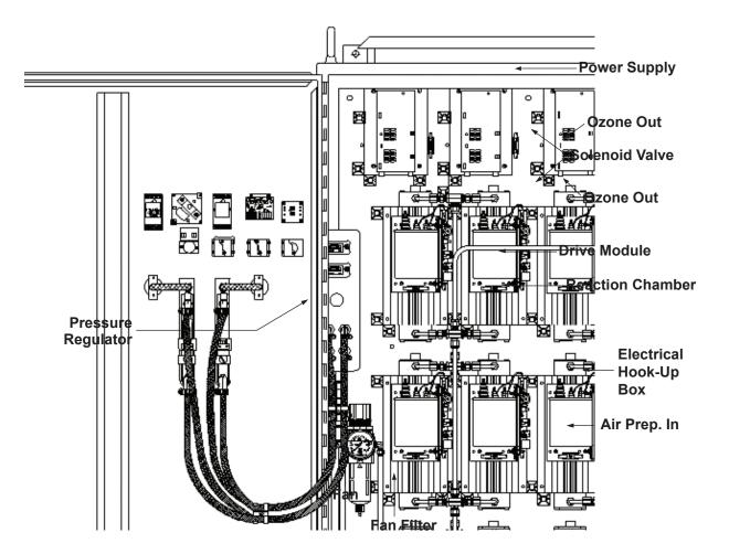
Shown: ClearWater Tech CD12000HO Ozone Generator (Wire harnesses omitted for clarity)
