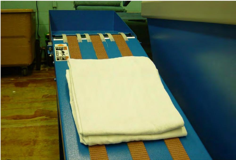
Figure 10. Hospital blankets being discharged from an automatic folder after ozone laundering.
