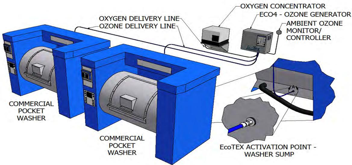
Figure 1. Schematic diagram of one of the three ozone system installations at the Gaston Memorial Hospital laundry facility.
