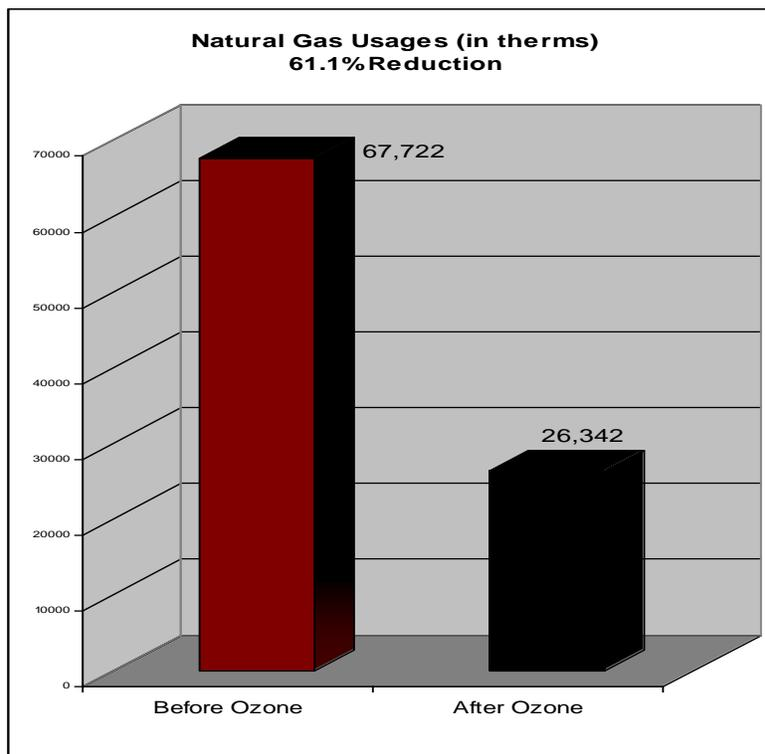
Figure 5. Natural gas reductions at Gaston Memorial Hospital due to ozone usage.
