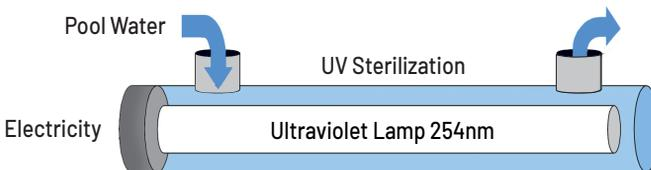
A properly designed, sized, and installed UV system will inactivate most microorganisms passing through it very quickly. Because of this, UV has been hailed as an ideal solution for pool water sanitation.
