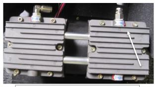
Compressor in Aerous 8, top view -Orientation is reversed in Aerous 15 -Pressure relief valve indicated by arrow
