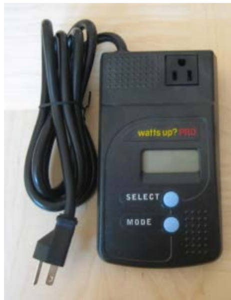
Figure 24. Watts Up Pro Power Meter (Photo: Navigant)
