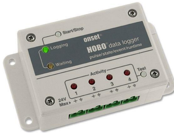
Figure 20. HOBO UX120-017 Data Logger (Photo: Onset)
