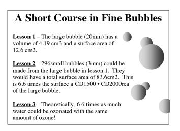
Depending on the application and the water treatment goals, a ClearWater Tech contacting system may also be required. Some oxidation reactions take place so quickly that they are limited only by the rate at which the ozone is dissolved in the water. Other reactions, such as disinfection, may require that proper ozone residual be maintained for a specific amount of time. A correctly-sized contact vessel is used for this purpose.
