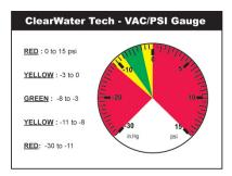
on the vacuum (in.Hg) side of the gauge, gradually open the ball valve on the injector manifold until the needle moves into the green zone. While vacuum is in the green zone you must be able to achieve proper SCFH (Standard Cubic Feet per Hour) of air flow (see the "Pneumatic Operating Parameters" chart for venturi SCFH required, Figure 10).
