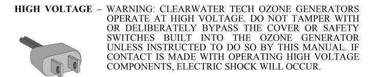
ClearWater Tech corona discharge ozone generators take line voltage and convert it to 48 VDC. A high voltage transformer then boosts the voltage. Proper care must be used by a qualified electrician when making any internal adjustments or performing any maintenance procedures.
